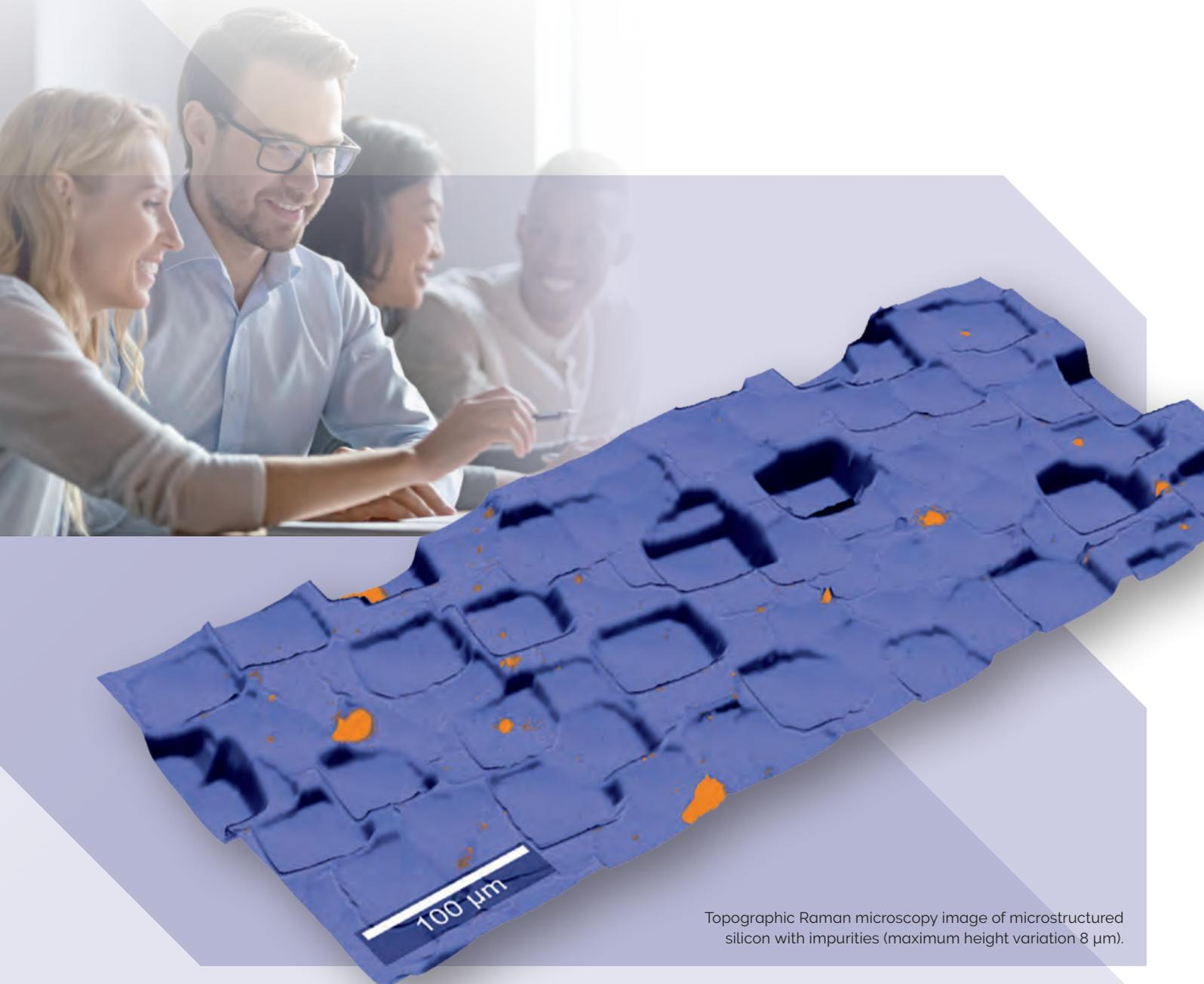
Topographic Raman microscopy image of microstructured silicon with impurities (maximum height variation 8  $\mu\text{m}$ ).
